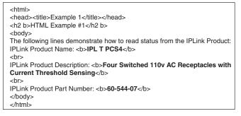
Figure 27. Resulting HTML Source Code Served by an IP Link web Server
